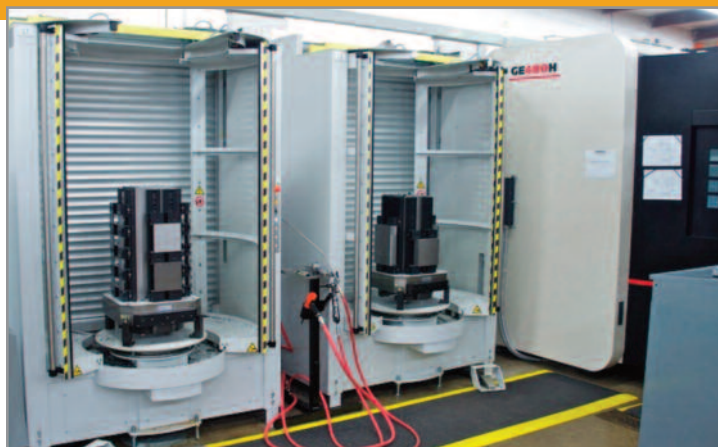
AME workholding tombstone devices on an Enshu HMC at TRD. 56 block sizes are run, producing over 450 different parts, in one-off to 500-piece quantities. The HMC runs in tandem with a Fastems 10-station (5 x 2) pallet changer.
