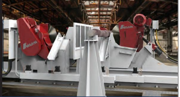
Heavy duty pivot saw to cut hot rail car axles.
