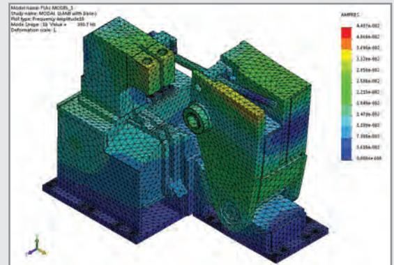
FEA performed on all machine designs to ensure stiff, vibration dampening machine structures and maximum tool life.
