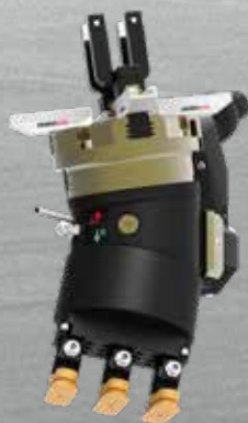
Smart Quad Grip system with two-point gripper and vacuum gripper
