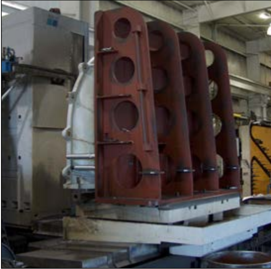
Image 2: The slurry pump housing half mounted on the fixture, mounted on a horizontal boring mill.
