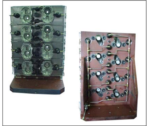
Front and back views of AME's dedicated hydraulic fixture for Southland CNC show the window feature that allows machining of all four sides of the part without additional handling.
