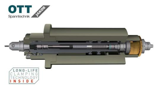
**02** PART CLAMPING FOR MACHINING OPERATIONS Similar to power drawbars, zero-point locating fixtures used in machining set-ups benefit from a power-off system. These clamping stations are pneumatically unclamped when shop air is introduced. When the workholding fixture is placed in position and pneumatic power is removed, the clamping stations activate to pull down on the retention knob offering extremely rigid and micron-precise clamping and locating for highly repeatable machining operations.
