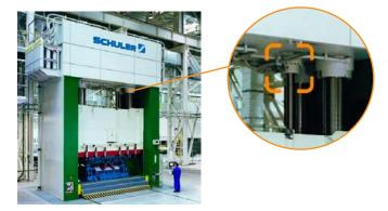
Sitema Safety Catchers are used wherever heavy lifted loads must be secured against falling or accidentally dropping. The Catchers are used where protection of personnel and accident prevention must be achieved. Catchers can control a falling mass at infinitely variable positions. Roughly 90% of safety catcher applications are for large industrial presses, which require a robust safety system.
