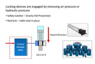
Unlike rod locks, where springs create the holding force, with the safety catcher the load itself creates the holding force so it is self-intensifying...no springs to wear or break. Instead, safety catchers utilize a tapered clamping system where the clamping force increases as the load increases.
