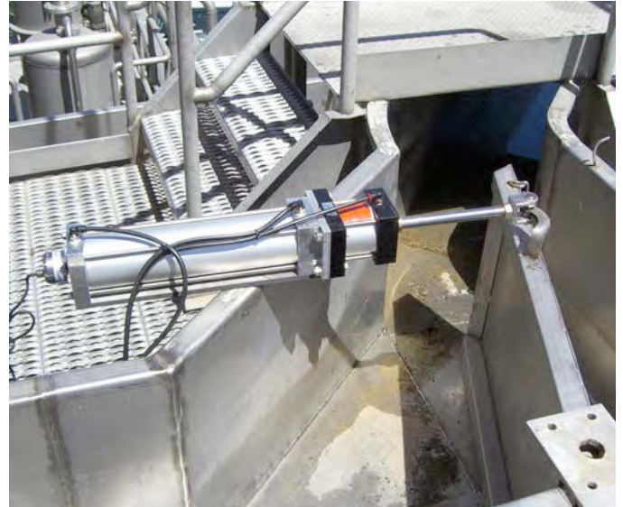
Amlok® RCN Pneumatic Rod Lock Application
