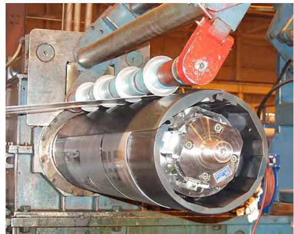
Aeromet mandrel shown with steel material rolled onto it; the drawbar taper is visible on the exposed end.
