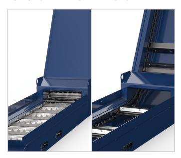
Our CDF technology achieves high levels of filtration without two separate belts. Our patented disc design provides a direct coolant flow path into the coolant reservoir and can filter a wide variety of materials, both in water and oil based coolant, down to 25 microns nominal, using a hinge OR a scraper belt.
