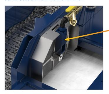
Self-cleaning permanent media with easy-to-access spary nozzles provide a continuous backwash spray that removes fines and chips, keeping the disc free from gunky build-up. No outside source such as air or steam is used.
