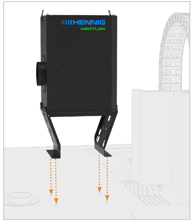
Fig. 5: Mounting on top of machine tool
