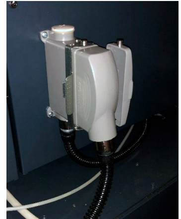
Female connector mounted to CNC enclosure, shown with male connector attached.
