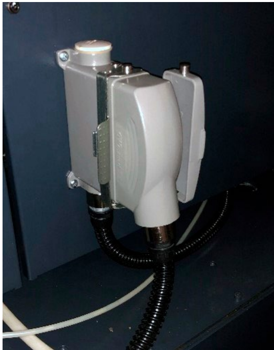
Female connector mounted to CNC enclosure, shown with male connector attached.
